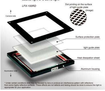
The LFX Series is a completely new type of light product enabled by CCS's cutting research and development capabilities. The pattern of dots on the surface of the light guiding diffuser plate controls light diffusion and transmission making uniform, omnidirectional light possible.
