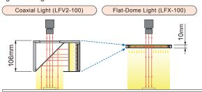
The LFX 100 requires 60-mm less installation height than the comparable standard LDM2-90 dome light with the same
